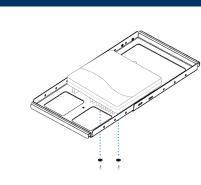
Now secure the CU to the **Ceiling Mount Accessory** using the two supplied **¼-inch Washers and ¼-20 x 5/8-inch Screws**.
